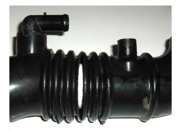
**Picture 4:** Flex hose with crack. We have put some white paper in the tube to make the crack more visible.
